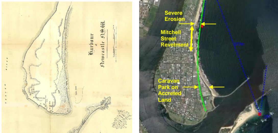
Figure 6. Left: Entrance to Newcastle Harbour (circa 1850). Right: Present-day entrance with MEPBAY 1850 predicted shoreline superimposed indicating foreshore re-alignment and severe erosion and accretion.
